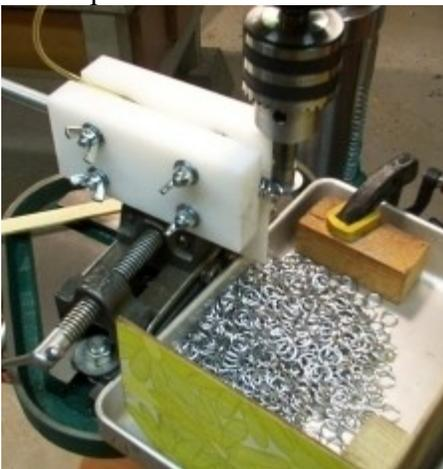
The block held in the vise, secured to the drill press table, will be referred to as the "vise block".
